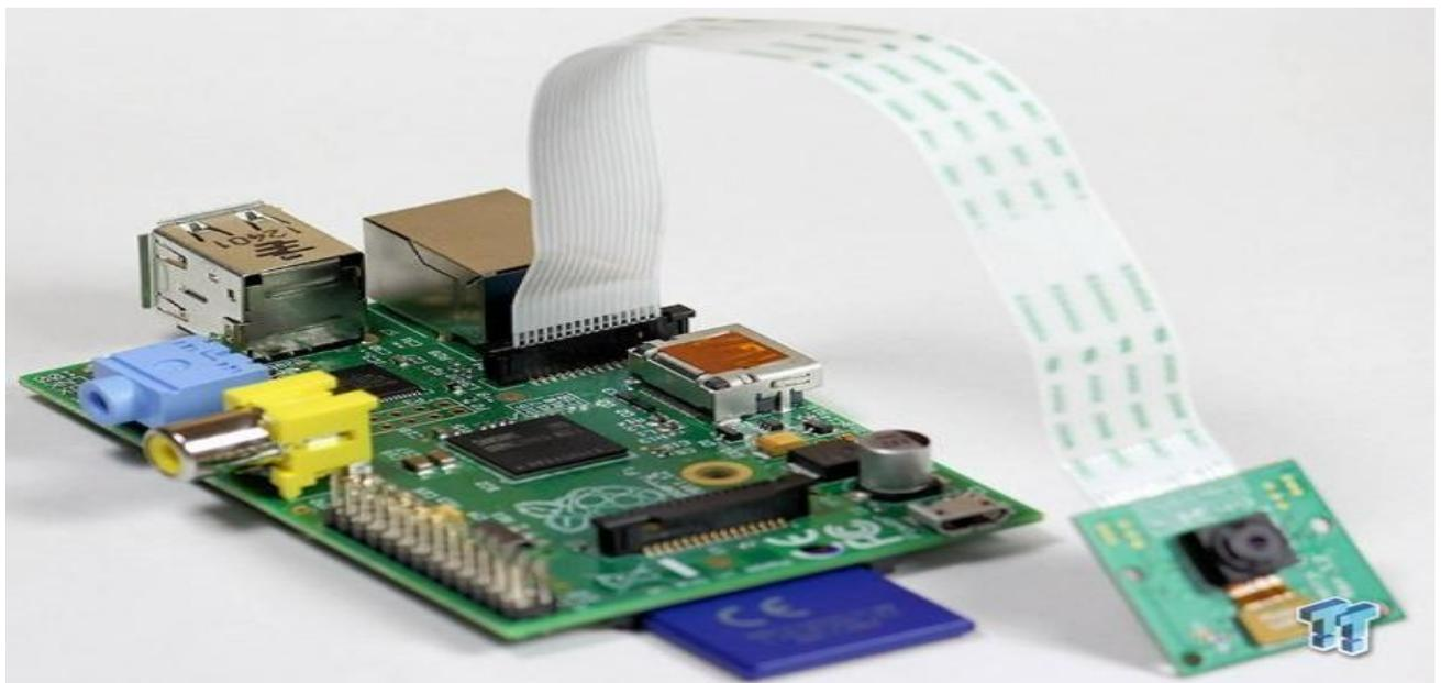
*Figure 3-26: Snapshot of Raspberry Pi camera module connected to Raspberry Pi*
