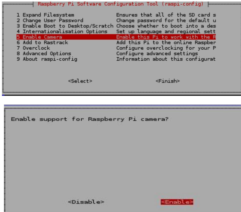
Figure 3-27: Snapshot of Raspberry Pi Camera Module installation in Raspberry Pi
