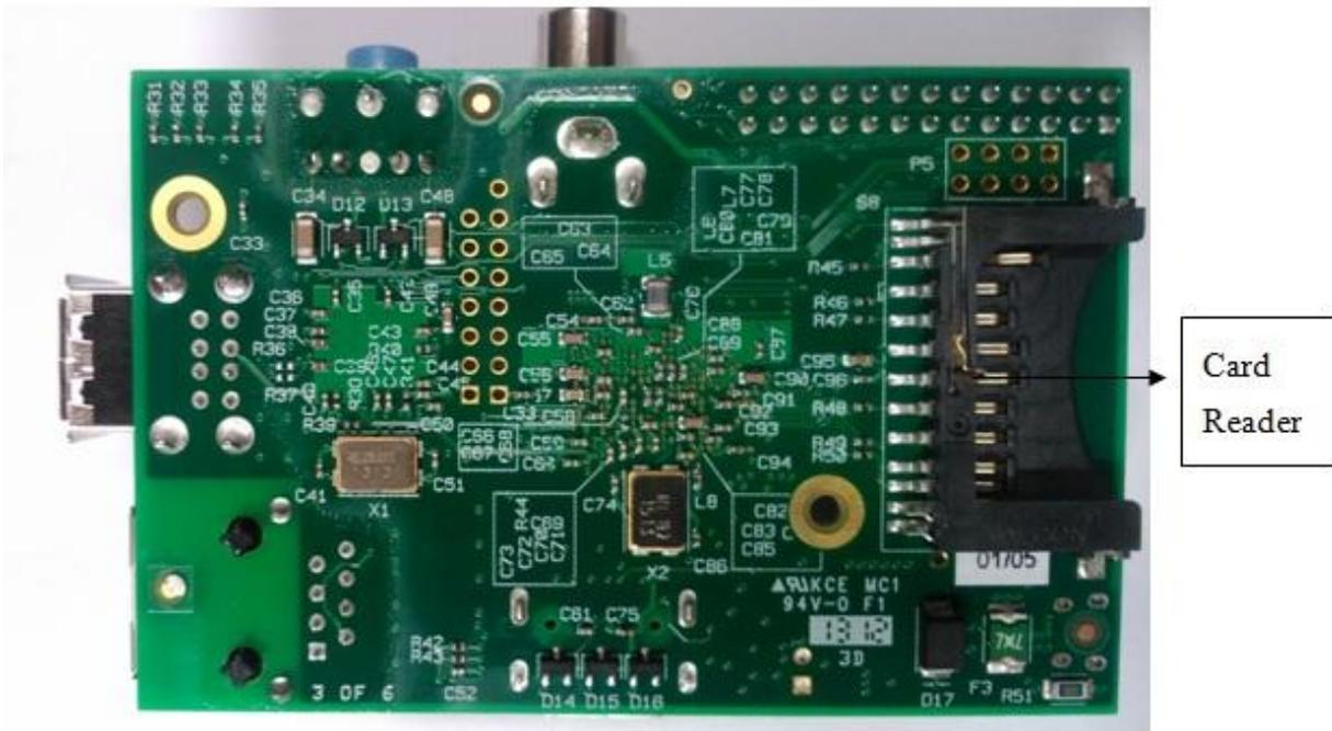
Figure 2-2: Back part of Circuit board of Raspberry Pi
