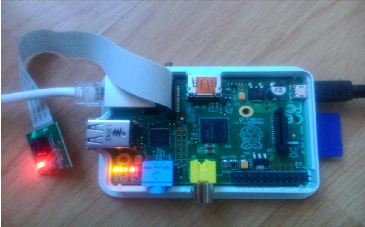
*Figure 4-16: Image of Raspberry Pi with Camera*
